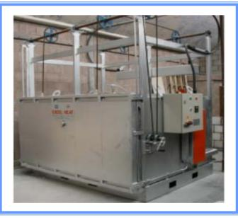
Unique Enamelling Services have invested in a new Excel Heat Ltd cast iron enamelling furnace specifically design for baths and cooker components.
